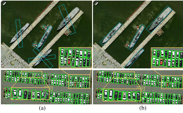
Fig. 4. Comparison of detection results between detectors with (a) smooth- L_1 loss and (b) RIL. (Top) Detections under OBB representation. (Bottom) Results under the QBB representation.
